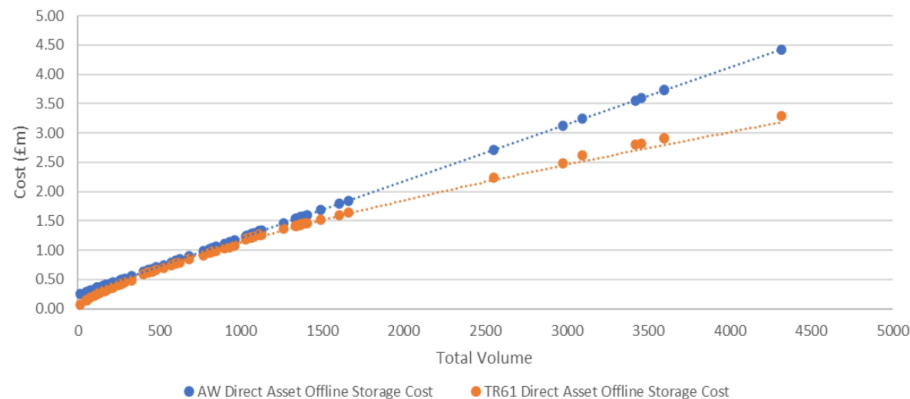
Figure 28 Benchmarking of concrete vs glass coated steel storm tanks direct asset costs
